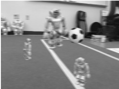
Figure B.6 – (Figure 3.3): Images programmatically generated by randomly combining the extracted isolation examples from Figure 3.2. Subfigure (a) shows images without any modification: the ball and robots are randomly scaled and placed. Subfigure (b) shows images that have motion blur added to the output image, as is typical of images taken from a roving robot. These modifications serve to enhance the realism of the final image, making the model perform better on real testing data.
