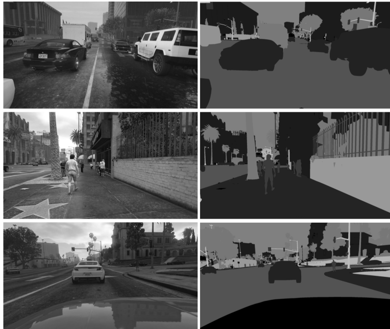
Figure B.1 – (Figure 2.2): Examples of video game footage and the associated classification labeling from Richter et al. Different colored pixels in the right images indicate different human-labeled classifications.
