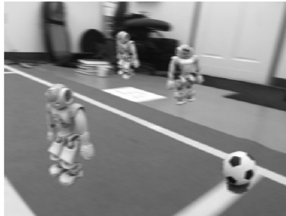
Figure B.6 – (Figure 3.3): Images programmatically generated by randomly combining the extracted isolation examples from Figure 3.2. Subfigure (a) shows images without any modification: the ball and robots are randomly scaled and placed. Subfigure (b) shows images that have motion blur added to the output image, as is typical of images taken from a roving robot. These modifications serve to enhance the realism of the final image, making the model perform better on real testing data.
