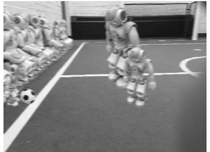
Figure B.6 – (Figure 3.3): Images programmatically generated by randomly combining the extracted isolation examples from Figure 3.2. Subfigure (a) shows images without any modification: the ball and robots are randomly scaled and placed. Subfigure (b) shows images that have motion blur added to the output image, as is typical of images taken from a roving robot. These modifications serve to enhance the realism of the final image, making the model perform better on real testing data.
